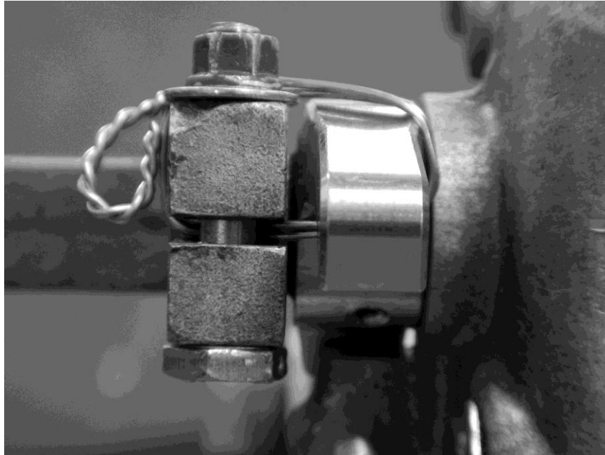
Figure 3-13c: Safety Wiring of Throttle Arm to Carburetor Stop Arm
