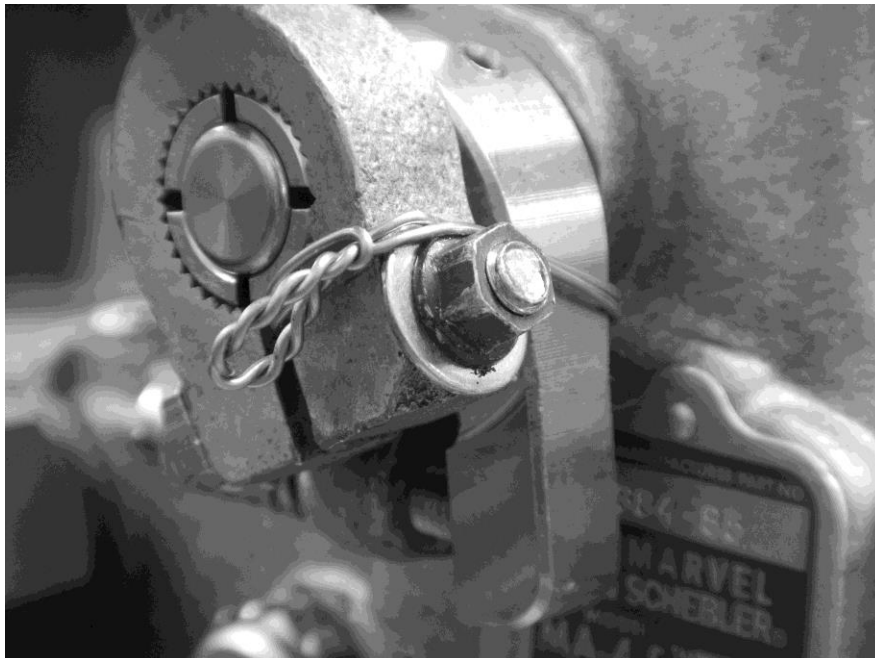
Figure 3-13d: Safety Wiring of Throttle Arm to Carburetor Stop Arm
